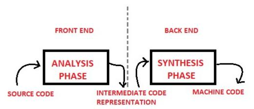
The code optimization in the synthesis phase is a program transformation technique, which tries to improve the intermediate code by making it consume fewer resources (i.e. CPU, Memory) so that faster-running machine code will result.
