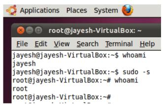
3) Can change the identity by using "su" command. "Su" command is used to change the user identity to another user. It is used as su – UserName. Use of "su" is shown in below image.
