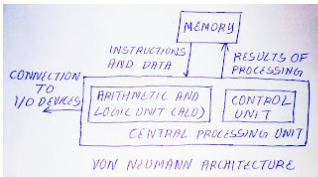
Computer architecture is based on Von Neumann Architecture.
